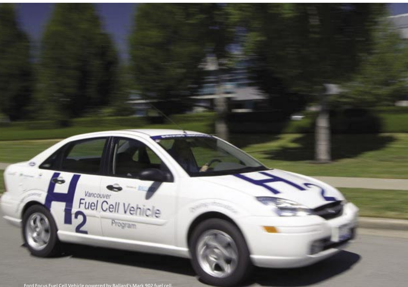
Ford Focus Fuel Cell Vehicle powered by Ballard's Mark 902 fuel cell. Cover Images Courtesy of: Angstrom Power, FCT, Ballard, Hydrogenics, Cellex Power.
