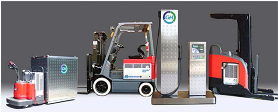
Figure 19 - Off-road Applications (courtesy of General Hydrogen).
