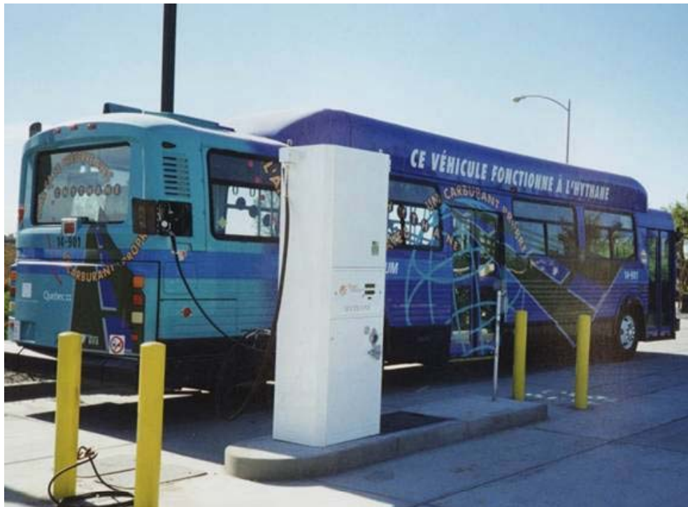
Figure 20 - Hythane ® Bus developed under Euro-Québec Hydro-Hydrogen Pilot Project. (courtesy of SunLine Transit).
